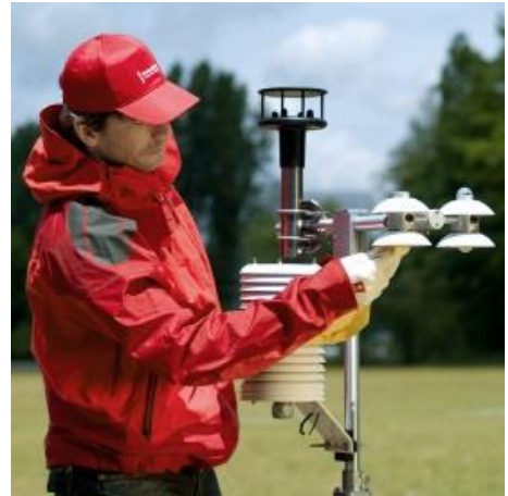
Figure 9 Measurement of net radiation to estimate regional evaporation of water [Hukseflux Thermal Sensors]
