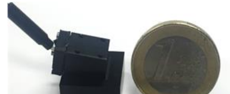
Figure 14 Dual-channel VIS-NIR spectrometer (350nm – 950nm), 1 cc including electronics. [Anteryon]
